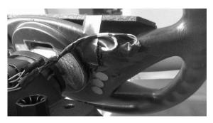
Figure 1. Force sensing resistors on steering wheel.
