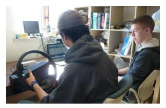
Figure 2. Participant (left) and experimenter. The participant's left hand is placed on the steering wheel, with his fingers on the FSRs.
